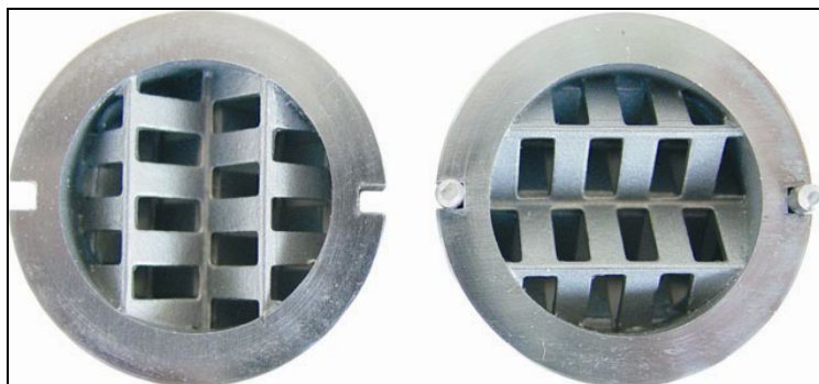
Figure #7: Adjacent SMN Mixing Elements are oriented 90^\circ relative to each other. Individual mixing elements can be separated and inspected from both sides.
